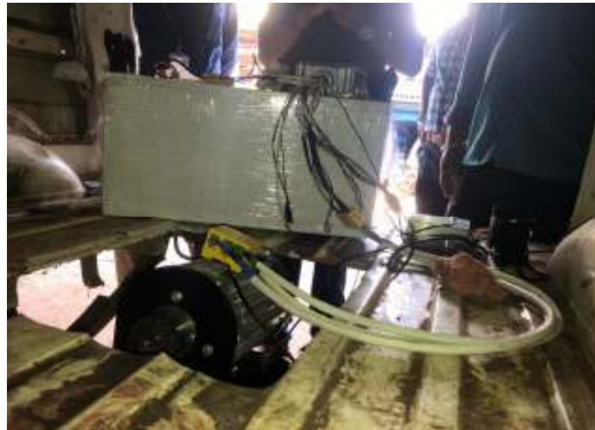
2. Assembly of Battery, Motor with the Rear axle
